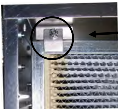
Figure 4. Close up of tabs for HEPA element
